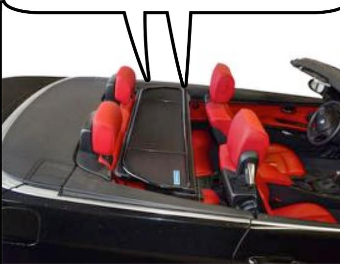
Start by extending the front and rear barrel bolts on one side of the wind deflector. Turn the handles so they will face down, this locks the bolts into place. These bolts will slide into the holes on the opposite side of the car from which you are standing.
