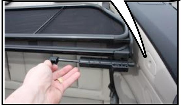
Next reach back and slide the rear bolt into the rear hole and turn the handle down to lock the barrel bolt.
