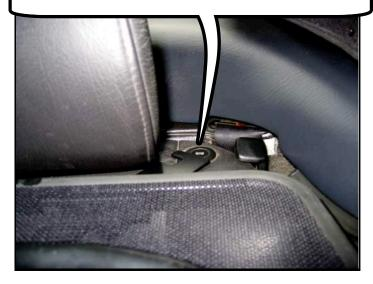
Make sure both brackets are locked into place on the headrest posts.
