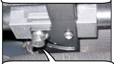
Tighten the lock nut on both sides. Turn the lock nut toward the drivers side to tighten and passenger side to loosen. The rear brackets will rest on the back seat.
