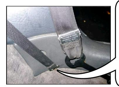
Attach the silver hook straps to the trim panel straight down, just behind the seat belt base. Then pull both straps down snugly.
