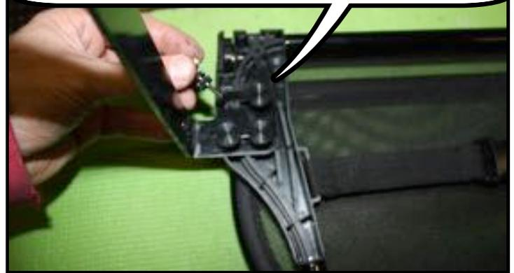
Lay the front brackets flat on the bottom of the wind deflector. The two thumb screws will go into the holes on the on the bracket and into the plastic. The other 2 will go into the plastic.
