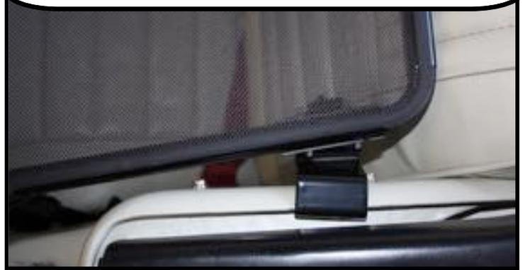
There are 4 straps that hold your wind deflector down. These straps are attached to the bottom of the rear trim panel.
