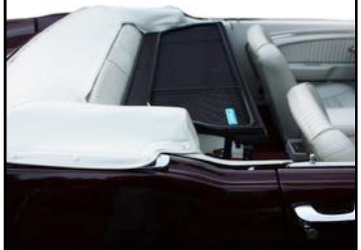
The front brackets are inserted into the Ash Trays in the back seat. Just slide the Ash Tray cover open and insert the front bracket into the front part of the Ash Tray
