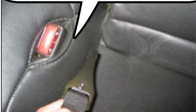
**Step 5 Cont:** The black snap hooks are inserted with the snap facing down. Slide the hook into the hole, press down and then pull back towards you to attach it to the anchor.
