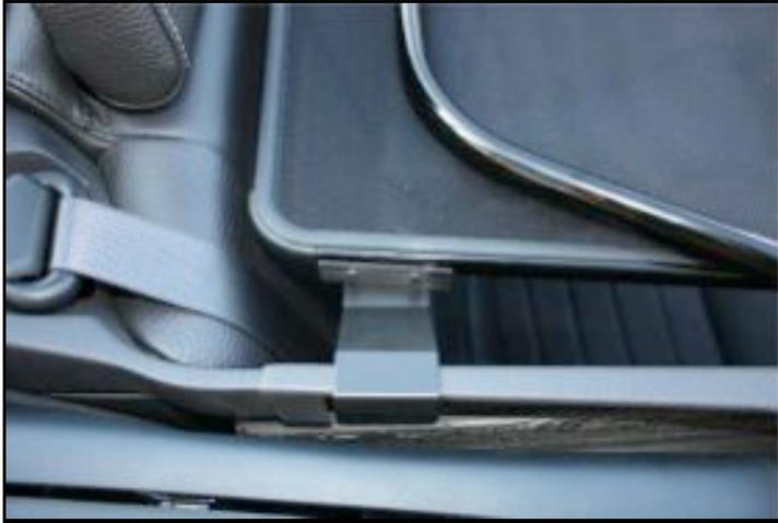
**Step 4 Cont:** The rear brackets may need to be adjusted so they fit tight against the trim panel. The adjustment is made by adjusting the two screws underneath the wind deflector.
