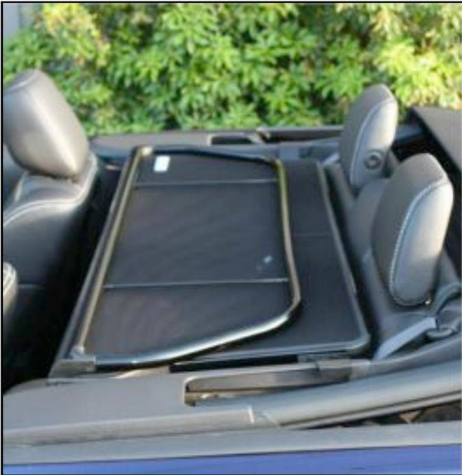
**Step 3 Cont:** The front brackets fit into the space behind the hole where the seat belt comes out of. The brackets are designed not to interfere with the seat belt.
