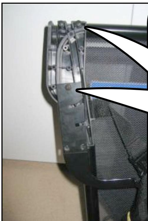
**Step 1:** When your wind deflector was shipped to you the front brackets had to be lowered to fit into the box. You need to remove the top two screws using a #2 philips (This is a very common screw driver and the end of the screw looks like an X) Do not remove the bottom screw.
