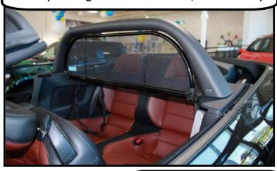
There are 4 straps that hold your wind deflector down. Two use the child anchor system and two attach to the bottom of the trim panel
