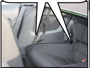
The black snap hook straps slide into the holes in the rear seats. They will lock into the Child Anchor system. Then buckle the strap into the wind deflector
