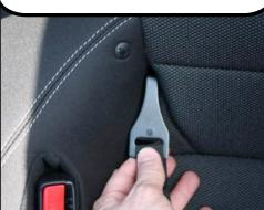
The silver hook straps hook into the cutout on the bottom of the trim panel and then buckle into the bottom of the wind deflector
