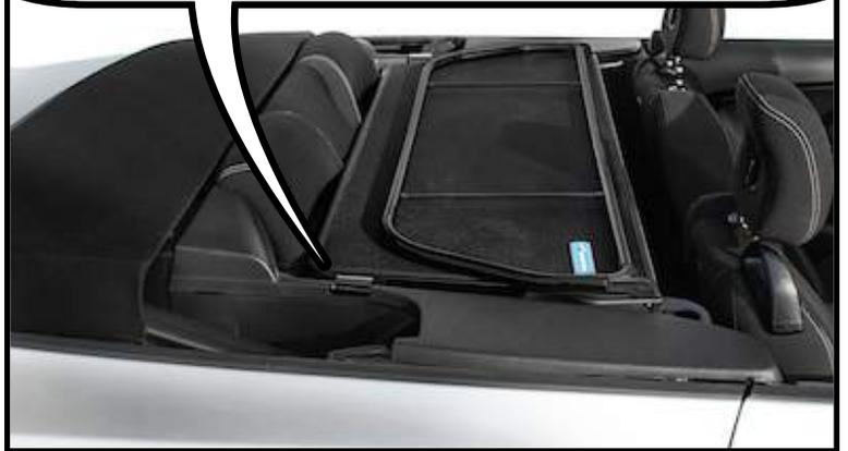
There are 4 straps that hold your wind deflector down. Two use the child anchor system and two attached to the bottom of the trim panel
