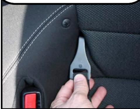
The silver hook straps hook into the bottom of the trim panel and then buckle into the bottom of the wind deflector
