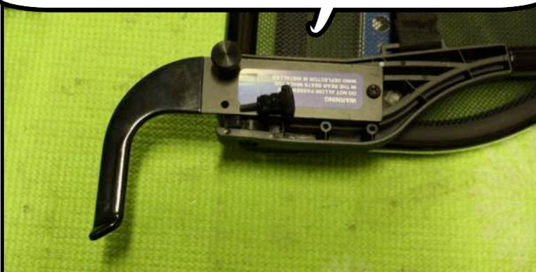
To store the wind deflector in the trunk remove the thumb screws from the front brackets. then turn the bracket down and store in the storage bag.
