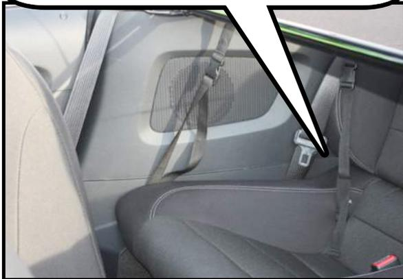
The black snap hook straps slide into the holes in the rear seats. They will lock into the Child Anchor system. Then buckle to the strap into the wind deflector
