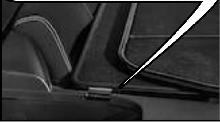
Start by lowering your top. Then lower the wind deflector into the rear seat area. Slide the front brackets into the seatbelt slots and let the rear bracket sit on the trim panel
