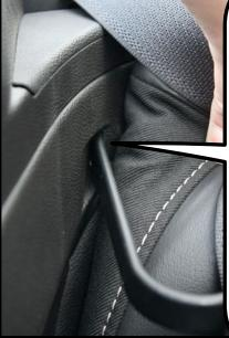
Now lower the wind deflector into the back seat area so the rear bracket goes into the slot beside the rear seat.
