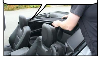
Next, flip out the rear bracket on your end and slide it into the rear slot. Now line up the
