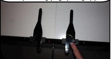
Lower the wind deflector into the back seat. Insert the extend barrel bolt into the hole on the trim panel, on the opposite side from which you are standing.
