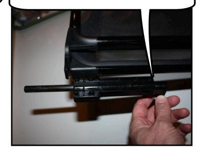
Loosen the thumb screws on the rear bracket (1 turn counter clockwise (Lefty = Loosey). Turn both of the rear brackets so they face out. Then tighten the thumbscrews by turning them Clockwise till they are snug (Righty = Tighty)
