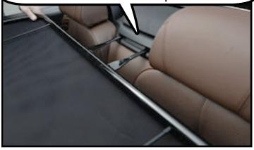
To easily store your windstop in the trunk you will need to lower the barrel bolts. Loosen (do not remove) the thumbscrew at the bottom of the barrel bolt. Remove the top 2 thumbscrews. Slide the bolt down and replace the thumbscrews in the top holes. Reverse the steps to move the bolt to the up position.
