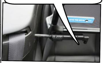
Complete the installation by closing the lid that covers your top completely. The rear brackets will be locked into place by lid and your wind deflector will sit securely in place.
