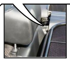
Now on the drivers side, while still holding on to the wind deflector, lower it so the barrel bolt is in line with the hole in the trim panel.
