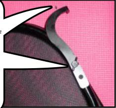
Standing on the drivers side of your BMW, insert the barrel bolt into the hole on the passengers side.
