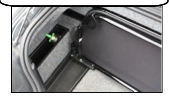
Then lower the wind deflector into the rear seat area so it is flat. The rear brackets will sit on the lip that is below the lid that covers your convertible top. You may need to adjust the rear brackets slightly inward to fit your BMW as each car is a little bit different.
