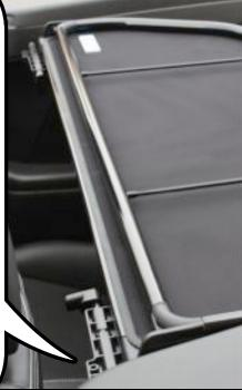
Then slide the plastic barrel bolt into the hole and turn the plastic handle downwards to lock it into position.
