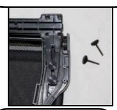
When storing you will need to fold in the rear brackets. Loosen the thumb screw by one turn (Do not remove these screws, only loosen)
