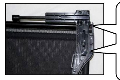
Start by sliding the plastic barrel bolt into the up position on both sides. The up position is when all of the thumb screws are below the bolt. Your wind deflector will arrive with the barrell bolts in the up position.
